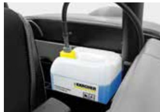
Cleaning agent dosing unit
