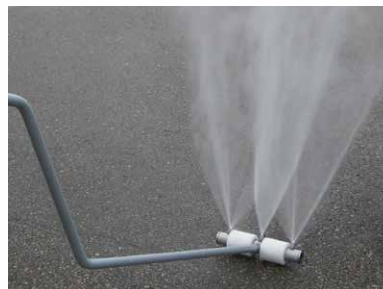
Rolling assembly keeps spray vertical
